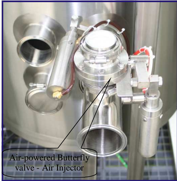
Large capacity 2" Air-Injector , with filtered air intake. Box of filters included.
