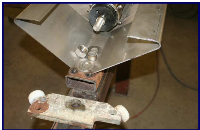
Old clevis shown in front. Center hole is too large for the 4" cylinder. Spacer bushing shown in the back ground
