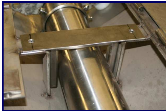
Adapter Bracket has two predrilled holes (nuts and bolts included). Drill new holes into the vertical legs of the original Germania brackets. As you already know, the original 5" cylinder was held in place with (2) bolts inserted horizontally and extremely difficult to get at.
