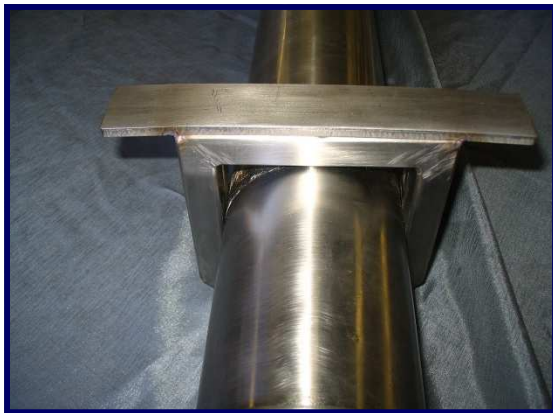
The new Cylinder comes with this adapter bracket to take up the extra space
