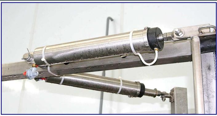
(2) Cow Traffic Controls at last stalls on either side of parlor. Plus (2) remote panels in front. 5-Button Crowd Gate controls on one side only. Stainless cylinders operate Entrance Gates & Automatic Indexing. Manual Exit Gates.
