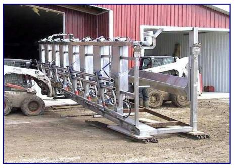
We build our parlor modules on platforms, a frame work made form 2" x 4" stainless tubing and usually 53" wide x 50 ft long for the typical dbl. 12. Normally, we slide the Modules into place on this steel frame work, pushed by a Skid Loader.
