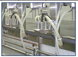
**HERITAGE** Top Outlet Claw hangs well balanced on the arm for milking and equally so in the rest position.
