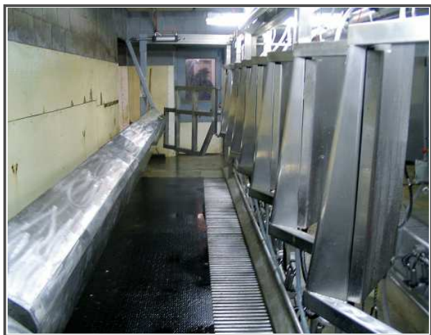
Auto-Indexing Brisket Bar, Grates, Gutter & Curbing, Slanted Splash Shields—everything 304 stainless
