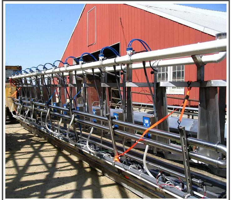
*The pit wall assembly contains all below-the-curb components. We rotate the assembly up 180 dgr. for transport - as shown here*
