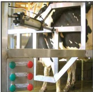
*Cow Traffic Controls with (8) new Cylinders, (4) for the Gates and (4) for automatic indexing*
