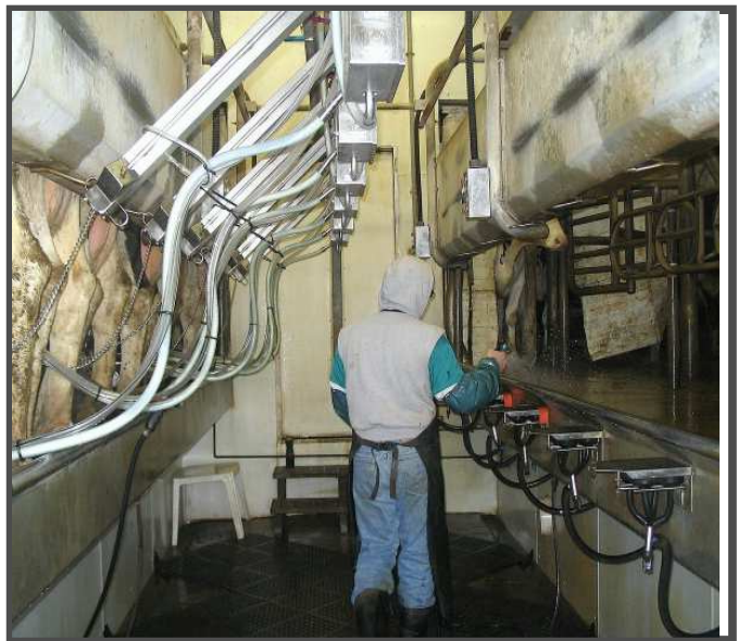
Wide open center - only the retract cylinder swings across the pit. Hoses swing with the cylinders
