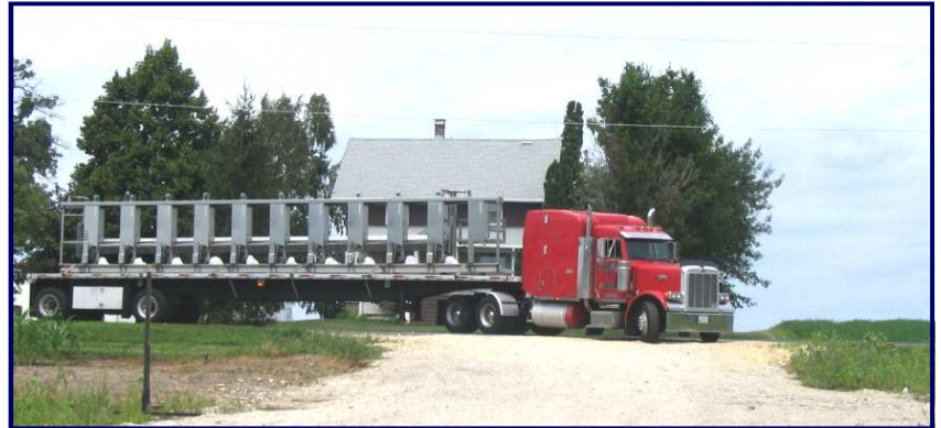
Parlor was pre-assembled in the factory and arrived at the dairy on two flatbed trucks
