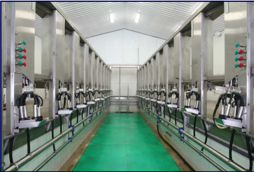
Dbl. 10 all-stainless HERITAGE ProTime I with Model SB Arm TakeOffs, Rapid Exit, Automatic Indexing and a Crowd Gate. Parlor planned for expansion to dbl. 16 later on.
