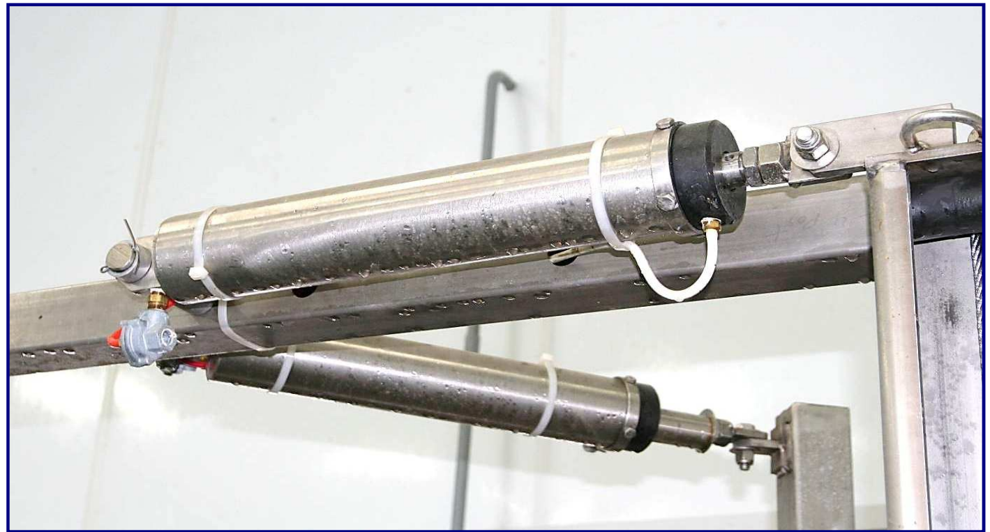
Cow Traffic Controls at last stalls on either side of parlor. Plus (2) remote panels in front. 5-Button Crowd Gate controls on one side only. Stainless cylinders operate all Gates & Automatic Indexing
